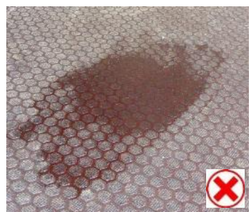
Oil contamination on Hexa Grip board over a length greater than 75mm.
