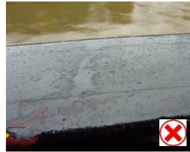
The original, intended slip-resistant paint coating on this narrowboat bow side deck has been degraded by the application of too much gloss paint over the original surface.
