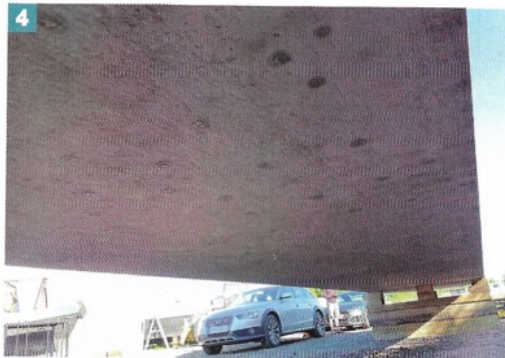
4 This base plate has been grit-blasted prior to survey at Droitwich Spa Marina.
